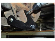
E. Install another  $\frac{1}{2}$  x 20 x 1  $\frac{1}{4}$  bolt with a 12mm flat washer on each side and torque to 70 foot pounds. The final should look like this.
