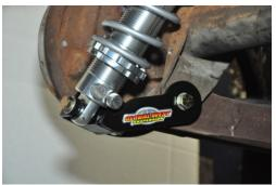
Adjusting the ride height is done by rotating the adjusting nut just below the spring. A spanner wrench included in your kit. The adjusting nut below the coil spring seat is a jam nut. The ride height is adjusted by turning the spring seat, Up raises the car and down lowers the car. Adjusting the ride height is best
