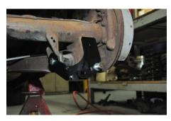
D. Use a drill with a ½ inch drill bit and drill a new hole through the differential lower arm mount.
