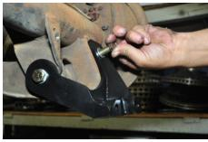
8. Install the shocks starting with the upper mount. Use a ½ inch x 20 x 3 1/4 inch long bolt with a 12mm flat washer and slide it through the upper shock mount. Next install one .315 spacer on the bolt.
