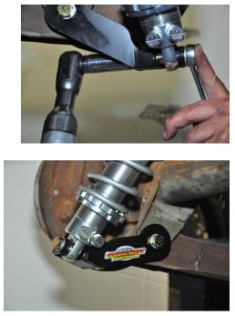
Adjusting the ride height is done by rotating the adjusting nut just below the spring. A spanner wrench included in your kit. The adjusting nut below the coil spring seat is a jam nut. The ride height is adjusted by turning the spring seat, Up raises the car and down lowers the car. Adjusting the ride height is best done by raining the car by the frame and removing tension on the spring and shock. After setting your desired ride height run the jam nut up to the spring seat and tighten.
