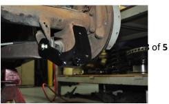
C. Install one  $\frac{1}{2} \times 20 \times 1 - \frac{1}{4}$  bolts with a 12mm flat washer through the hole that is aligned with the original shock mount hole. Tighten down the bolt to 70 foot pounds.
