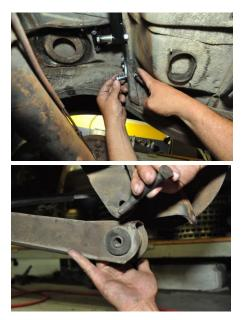
7. Install one of the new lower shock mounts using a
