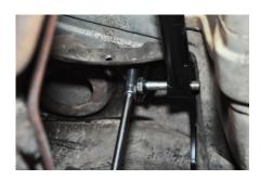
5. The cross member is now lined up against the frame, use a drill with a 3/8 drill bit and drill the frame for mounting the cross member. After the first hole install a 3/8 bolt and nut and just snug.
