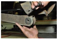
Install one of the new lower shock mounts using a new ½ x 20 x 4 inch bolt and one 12mm flat washer. Slide the bolt through the new lower shock bracket and differential. Install a 12mm washer and a ½ x 20 lock nut on the other side.
