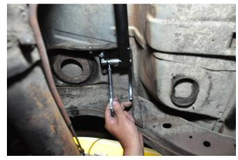
Once the cross member is lined up tighten down the shock mount bolts.
