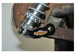
Adjusting the ride height is done by rotating the adjusting nut just below the spring. A spanner wrench included in your kit. The adjusting nut below the coil spring seat is a jam nut. The ride height is adjusted by turning the spring seat, Up raises the car and down lowers the car. Adjusting the ride height is best done by raining the car by the frame and removing tension on the spring and shock. After setting your desired ride height run the jam nut up to the spring seat and tighten.
