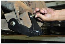
8. Install the shocks starting with the upper mount. Use a ½ inch x 20 x 3 ½ inch long bolt with a 12mm flat washer and slide it through the upper shock mount. Hold the shock in place and slide the bolt
