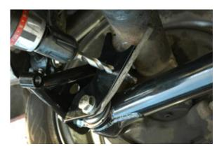
16. Now install the upper cross brace to the frame. The shocks should already be removed. The brace will
