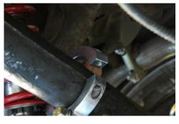
22.Locate 2 allen head bolts and place a little red loctite on the threads. Swing the clamp up so it sets flat
