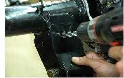
13. (On the Bench) --- Next if you are doing this on the bench, you can drill the side hole now or install the tubular support bracket. In this case we drilled the hole with the bracket out of the way. Using a ½ inch drill and ½ inch drill bit, drill the side mounting bolt hole. Make sure the bracket is tight
