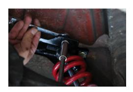
19. Install the lower portion of the shock. Locate a 5 inch long ½ inch bolt and slide it through the tubular lower mount. Install one of the tapered shock mount spacers first on the bolt. The taper
