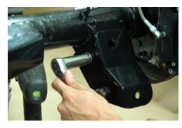
(On the Bench) --- Now install the tubular support bracket. Use a  $\frac{1}{2}$  x 20 x 2  $\frac{1}{2}$  bolt with flat washer and slide it through the mount. Use a thick wall  $\frac{1}{2}$  inch flat washer with a lock nut and slightly run the nut down a few threads just to hold the bracket in place.
