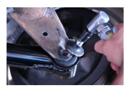
10. Locate in your kit one of the 5/8 bolts with a flat machined into it. Slide a flat washer on it and install the bolt through the correct (right or left) shock mounting bracket supplied in your kit. See photo -- You can run the new lock nut down but do not tighten the bolt yet.
