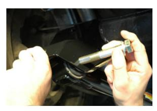
11. (On the Bench) --- First you are going to position the lower support bracket on the rear end. Slide one of the new bolts with a machined slot through the new bracket and lower arm bolt hole on the rear end. See photo. Next tilt the bracket up tight against the rear end and use a 5/8 jam nut provided in your kit tighten down the bolt enough to hold the bracket tight up against the rear end.
