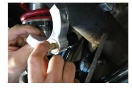
21. Next install the aluminum clamps that go around differential. The lower clamp has locating hole for the lower shock support tube. Use a 2 inch ½ inch
