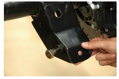
12. (On the Bench) ---Your rear end may already have an upper hole in the bracket. If not you will have to drill one. Drill the upper mounting hole to ¾ of an inch.
