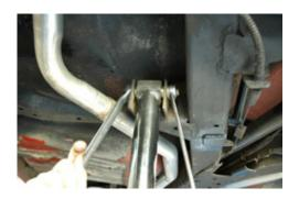
rear end side. New hardware is supplied. The front of the arm has a special bearing in it that allows for pivot. Install the front of the arm on the frame first. It has a spacer on each side of the bearing. They are already installed in the arm. Make sure the spacers don't fall out during installation; you will need them for proper spacing in the frame bracket. Tighten to 120 foot pounds.
