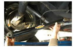
9. Before installing the rear arm on the rear end side check the new bracket fit to the rear end. You may have to buff the lip on the rear end bracket so the coilover bracket sets flat along the side.
