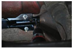
17. Once the cross member is bolted in, use a ½ inch drill motor with a ½ inch drill and drill an additional bolt hole through the frame. One on each side of the cross member.
