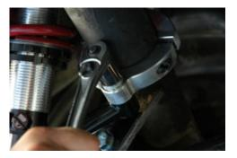
23. After the clamps are tight, tighten down the bolt holding the short shock support tube.
