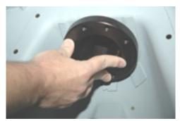
3. If you have ordered a negative roll system you will have an upper control arm template for drilling different locating holes. Note: If you did not order a negative roll system no template will be provided but you will have to drill the upper mounting holes out to 9/16 diameter. The original holes are ½ inch diameter. Slide a couple of ½ inch bolts through the template and inner shock tower.
