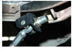
the frame. Occasionally due to frame discrepancies the hex adjuster may need to be lengthen or shortened in order for the arm to
