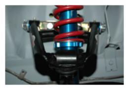
9. Rotate the upper mount till it sides through the shock tower hole. Once the allen bolt gets past the tower you will be able to index the mount. Install the mount using the hardware supplied in your kit. Tighten down the bolt to 25 foot-pounds. Note: You do not need a cushion between the billet mount and the shock tower.
