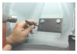
Drill the new hole location with a 3/8 drill bit and then step the hole up to a final size of 9/16 diameter.
