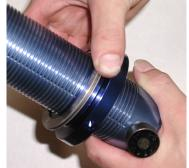
C. Slide the needle bearing assembly onto the shock adjuster.
