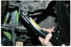
Important – (Adjusting the lower arm). With the control arm bolted tight to the chassis, cycle the lower control arm up and down making sure it moves freely. With a 1-inch wrench, adjust the hex adjuster so there are approximately two threads showing on each side of the jam nuts. Feel
