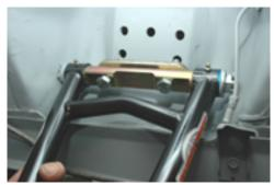
the 3/8 inch steel spacer plate between the upper control arm shaft and the shock tower. If you do not have a negative roll system you will not have the plate. Just bolt the upper control arm direct.) Just tighten the nuts down. Do not torque them down because the alignment is going to be done using shims between the upper arm and shock tower.
