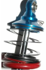
bearing. Slide the allen bolt through the mount with one spacer on each side of the bearing. The allen bolt nut indexes on one side so you do not need a wrench to hold it. Simply start the bolt and tighten down to the nut. The nut just needs to be tight no set torque is required.
