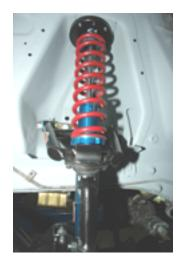
13. Install the new inner tower supports. The stock support would bolt on as seen in the photo to the left. The tubular support installs just as stock. There is a right and left unit. You cannot install them incorrectly. Hardware is supplied.
