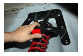
Install all the bolts and nuts in the support loosely. Place the head of the bolt in the engine compartment side. Tighten down the top 2 bolts first and then move from the top, side bolts down the bracket. Tighten to 25 pounds.
