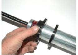
The photo to the left shows a QA-1 application with jam nut.
