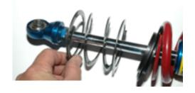
G. The upper cone slides over the shaft as shown to the right.
