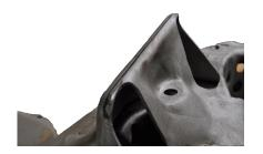
2. Next mark the welds that hold the shock plate on the frame. You are
