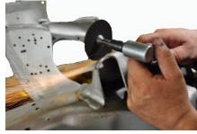
Right: Cut the welds off holding the shock plate.
