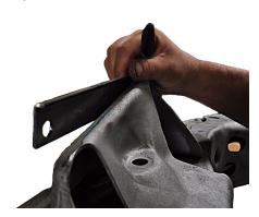
Take a marker and trace the edge of the plate along the top of the frame. This is your cut line.
