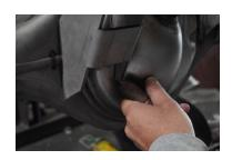
If the measurements check out, weld the bracket to the differential. When you are done welding you should be able to slide the 5/8 rod through the upper arm holes with no problem.
