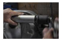
Take the new bracket and run a bolt through the bracket and into the other side of the aluminum bar. We install another rubber bushing in the bracket. This will set the correct distance across the rear end for the new bracket. Check to make sure the bracket fits nice up against the differential housing. You may have to do some grinding for a good fit.
