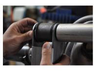
The fit should be so the aluminum bar is parallel to the axle and the same distance from centerline of the axle. A few quick measurements will verify. Once you are pleased with the position tack weld the bracket to the differential.
