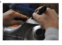
Next move the ruler a little lower and mark the differential in order to establish a line. The bracket will line up on this line.
