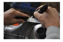
Next move the ruler a little lower and mark the differential in order to establish a line. The bracket will line up on this line.
