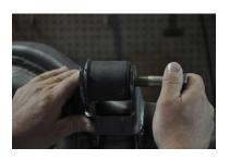
Next thread one end of the aluminum bar onto the bracket.
