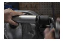
Take the new bracket and run a bolt through the bracket and into the other side of the aluminum bar. We install another rubber bushing in the bracket. This will set the correct distance across the rear end for the new bracket. Check to make sure the bracket fits
