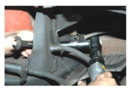
3. Locate in you kit new hardware (3-7/16 bolts). The bolt head with a washer should be on the bracket side for stock upper control arms. In this case during installation Global West used shorter bolts in the picture because **Part # TBC-94** was being used. In your kit, longer bolts are furnished
