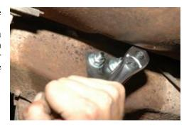
3. Re-install the upper control arm. Use the new 5/8 bolt supplied in your kit. Place a flat washer on first and slide the bolt through the upper hole in the bracket. **This is the only hole you can use if**
