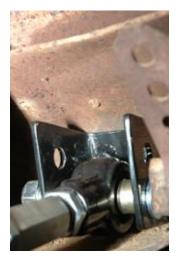
you are using a stock upper control arm. If you are using Global West's Part # TBC-51, install the arm in the lower hole. Use a 5/8 flat washer, locknut and torque to 90 footpounds on the frame side only. Do not torque the rear end side till the rear suspension is fully loaded. If you are using a stock upper control arm you cannot torque either side till the full weight of the car is resting on the rear end.
