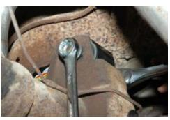
4. After you completed tightening down the bolts, the installation is complete. The finial step will be to re-adjust the pinion angle if you are using Part # TBC-51. If you are using the stock control arm, you would reuse the shims and recheck the pinion angle.
