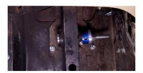
12. Once the bushing has bottomed out, release the tension on the bushing and unthread the plug off of the rod. You will have to thread the rod deeper into the housing so threads protrude at least  $\frac{1}{2}$  an inch past the frame. Flip the threaded plug around and thread it back onto the rod. Retighten the nut and finish pulling the bushing into the frame. The bushing will stop when it contacts the threaded plug and will be flush with the frame.
