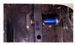
11. Using a % wrench, tighten the nut, the bushing will pull into the frame hole. Wrench the bushing in until it bottoms out on the threaded plug.
