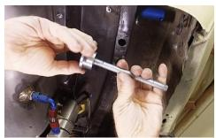
7. Slide the assemble from the inside through the frame and bushing on the passenger side. The driver side rod will slide through from the outside and you will thread the rod into the steel plug when it is in the housing. This is because of the gas tank.
