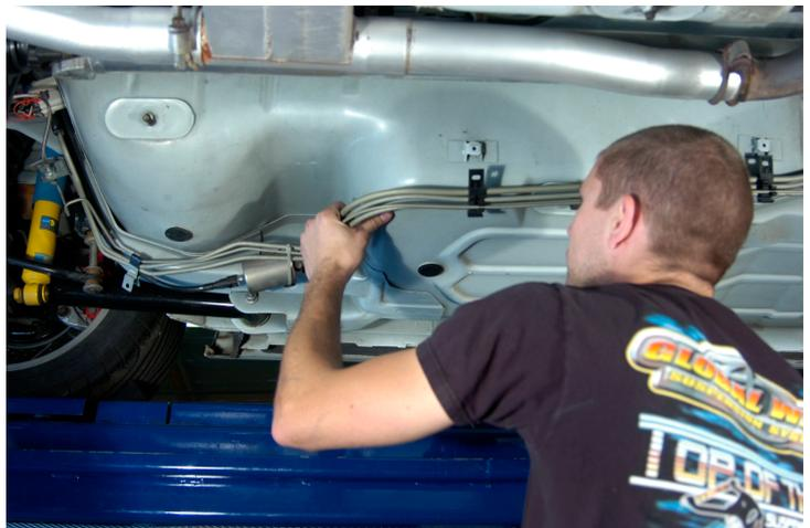
4. Once the lines are loose, remove the rear seat cushion behind the driver seat. Next remove the rear seat belt and bolt which screws into the drive shaft tunnel. This allows you to obtain clearance to get underneath the carpet in that area.
