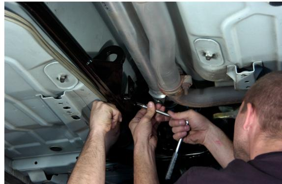
13. Next install the exhaust bracket. Using the 3/8 bolts, flat washers and lock nuts, re install
