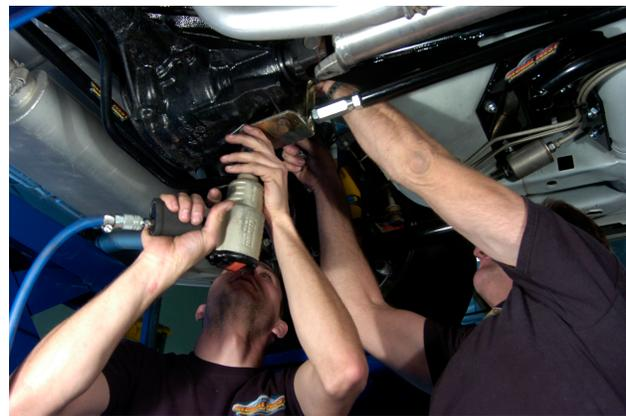
16. At the front of the torque arm you need to finish installing the collar. Locate the other rubber bushing and slide it onto the collar. The flat portion goes on first with the tapered part of the rubber bushings towards the front of the car. Install the concave flat washer next. The curve of the washer goes towards the rubber bushing. Install the 1 inch jam nut and tighten down the nut until there is about 3/8 of an inch on threads showing.
