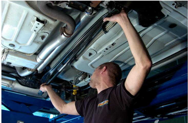
3. Once the torque arm is removed unbolt the little clamps that hold the brake lines and fuel lines. These lines run down the center of the drive shaft tunnel. The fuel filter must also be unbolted from the frame. **DO NOT UNDO THE FITTINGS ON THE FUEL LINES OR BRAKE LINES.**
