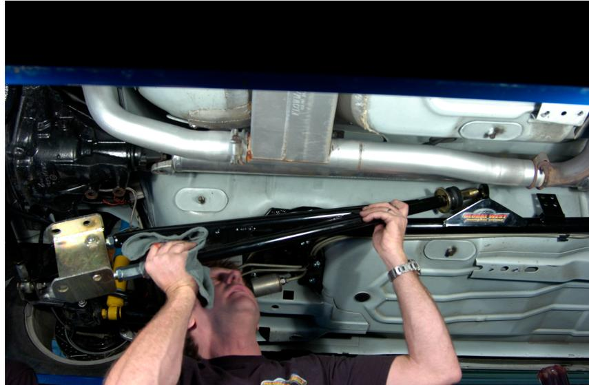
15. Swing the back of the torque arm up onto the rear end and slide the factory bolts through the assembly. You may have to raise or lower the body in order to get the torque arm bracket onto the rear end. Tighten the bracket to the rear end to 90 foot pounds. Torque the two bolts holding the torque arm to the bracket to 65 foot pounds. They are located on the side of the bracket.
