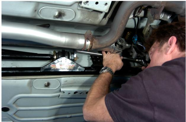
21. With the vehicle back on the ground recheck pinion angle. (You must check the pinion angle with the car on the ground or at least the suspension loaded as if it was on the ground.)
