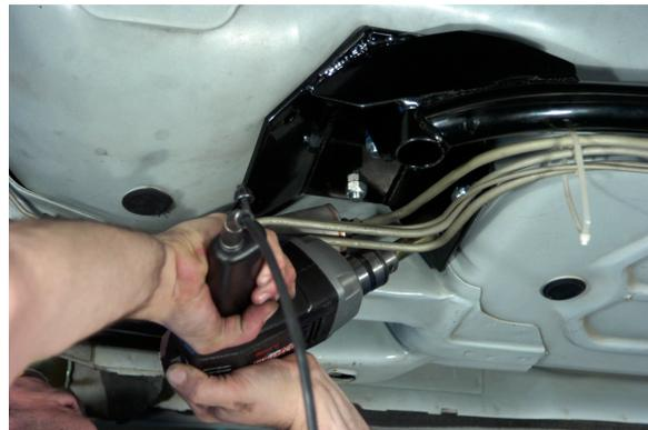
12. The Traclink main beam is now installed; you may put back the fuel lines and brake lines. The lines may require slight bending to get them back into position. This does not need tools, just bend them with your hands.
