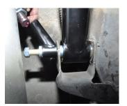
Above photo shows spacer required ----- spacer installed ----- longer bolt requires
