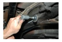
4. The frame support will also require prepping. Take the small grinder and buff the powder coat off the sides of the angle tab.
