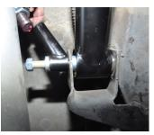
Above photo shows spacer required ----- spacer installed ----- longer bolt requires
