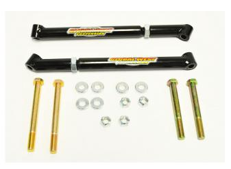
kick off the bottom of the lower control arm mount. Spacers are provided so you can align the brace properly without putting the bolts in bind. It is possible that the spacer maybe used on the top or bottom. Basically where ever the combination is required.
