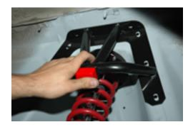
4. Install all the bolts and nuts in the support loosely. Place the head of the bolt in the engine compartment side. Tighten down the top 2 bolts first and then move from the top down on the bracket. Tighten to 25 pounds.
