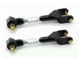
the adjuster. Adjusting one end only will offset the amount of threads required for holding the arm together when installed on the car.
