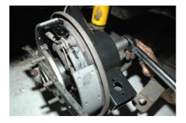
21. Install the strut rod and shock.
