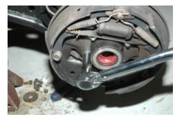
Install the 7/16 flat washers and lock nuts supplied in your kit --- Torque to 65 pounds.
