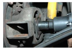
need to tap the assembly out with a dead blow hammer. Doing it this way is cumbersome because the enter assembly is being handled all at once.
