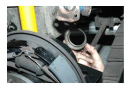
20. Install the axle shaft steel thrust washer, castle nut and torque to 120 foot-pounds. Install the axle ½ shaft and torque to 65 footpounds.
