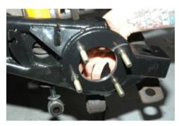
13. Next install the hub. You will notice the hub is separate from the brake assembly. We always service the bearings when installing a new swing arm. Therefore the assembly is apart as shown.
