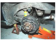
3. Remove the spring bolt and cushions. Note in this particular case the bolt is not factory and the head of the bolt have been machined round. In order to remove the bolt a vise grip is required. Once you have
