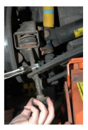
5. Remove the strut rod and the shock from the swing arm.
