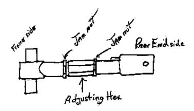
on the ground fully loaded. Adjusting the length of the arm is done simply by rotating the adjusting hex. After the pinion angle is adjusted to your specifications, tighten down the jam nuts while holding the adjusting hex from turning.
