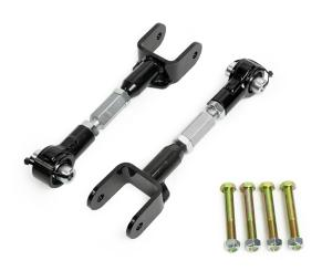
the length of the arm by placing a wrench on the adjusting hex sleeve. This is approximately two inches long located between the jam nuts. Rotating the adjuster will change the length of the arm. **DO NOT** adjust one end of the arm by itself! Use the adjuster. Adjusting one end only will offset the amount of threads required for holding the arm together when installed on the car.
