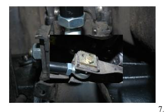
Next swing the strut rod up into the bearing hub. Make sure the 5/8-inch steel spacers are still in the
