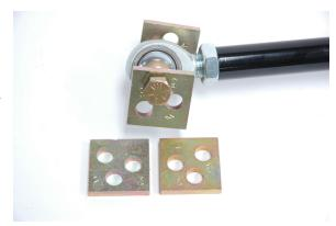
When installing the plates in the rear end bracket from the rear looking forward --- use the bottom hole about in the middle of the plate. # 3 You will be able to read it. Place the ½ inch bolt supplied in your kit through the plate. Take the strut rod (the side with the steel sleeves with ½ inch hole in them) up into the bracket. Slide the bolt through the enter assembly.
