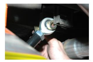
6. Next install a plate on the other side of the rear end bracket. Again in the #3 position. Install a  $\frac{1}{2}$  x 20 self-locking nut and torque to 70 foot pounds.
