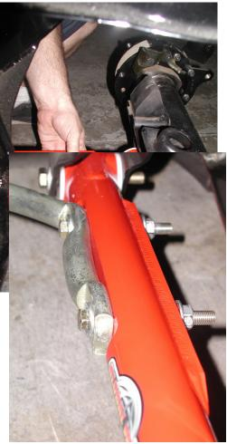
Torque the sway bar to frame bolts to 45 foot pounds.
