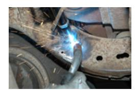
9. After welding the support on the passenger side. Weld the driver side in the same fashion
