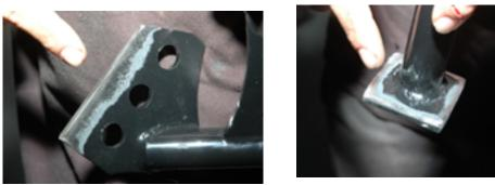
Buff off the powder coat around the 3-bolt bracket along the backside edge and top. Buff only what you see in the pictures.
