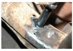
Weld all around the support pad to the frame.
