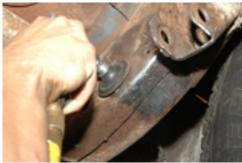
While you are buffing off the frame, buff off the side of the track bar frame bracket along the sides and top area.
