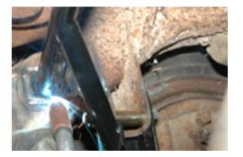
10. Once you have the support brace welded, buff the backside of the track bar bracket and a little of the frame. See photo to the right.
