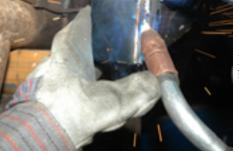
Also weld along the top of the new track bar bracket to the original frame bracket.
