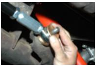
4. The jam nuts should be loose at the hex adjuster. Using a tape measure, pick a point on the fender well opening and measure to the tire. Go to the other side of
