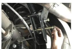
assembly. Next install the 9/16 bolt through the lower 2<sup>nd</sup> hole in the bracket. You will require using one of the steel sleeves (spacer) furnished in your kit. As you install the bolt through the bracket and frame mount, place the steel spacer in the middle and slide the bolt through. This will keep the bracket from distorting when you eventually tighten the bolt. At this time you can tighten the two  $\frac{1}{2}$  inch bolts holding the new bracket and cross brace (70 foot pounds).
