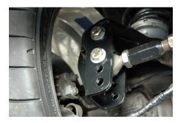
18. The track bar is adjustable for centering the rear end in the chassis. Simply loosen the jam nuts on the adjuster and rotate the adjuster till the rear end is centered and then retighten the jam nuts. Installation is complete.
