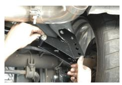
After you have the bracket capable of being installed so the holes line up, you will have to open up the top hole using a ½ inch bit. The lower hole will require using a 9/16 drill bit. Both holes will require drilling.
