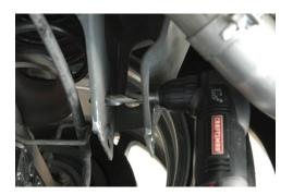
5. After the holes are opened up, install the bracket and the upper cross brace. Line the new bracket up on the frame mount and slide the upper bolt through assembly. Using the ½ inch bolt provided in the kit. The brace will line up with the original mounting holes on the body. Install the three upper bolts and tighten them down. Do not tighten the 16
