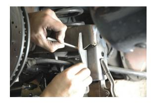
Weld the gusset to the rear end and bracket.
