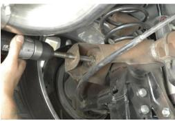
10. Install a 9/16 bolt and washer through the bracket and using the other 1 7/8 spacer from your kit, place it in the middle of the mount and slide the bolt through. Do not tighten it down all the way.
