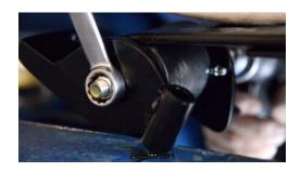
6. Use the floor jack and raise the differential with leafs attached. Slip the mounts into position over the studs. There is a small tab that indexes in the unibody located on the flat plate next to the forward bolt. That must index in the slot.
