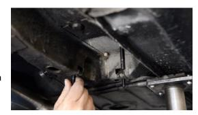
Install all the studs into the factory clip nuts at this time.
