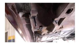
6. Remove the stock mount off of the leaf spring. Locate the correct lsb-71 mount for the side you are working on. The lsb-71 mount has a tube welded to one side. This goes to the outside of the car. The long stud indexes in the tube. First determine which hole you are going to use in the mount. If you are using our reverse eye spring you will use the bottom hole. Do not raise the leaf up to the top hole. If you are using a standard eye leaf spring, you can use either locating hole.
