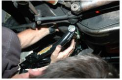
Index the upper part of the spring first and then swing the lower arm up to the spring. Rotate the spring cushion until the cushion will index with the spring. Use a floor jack under the lower control arm help hold the arm close to the spring. The floor jack should be positioned towards the ball joint side, not directly under the spring pocket.
