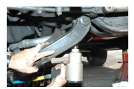
lower control arm up against the frame and install a 9/16 bolt with large flat washer through the hole in the frame from the top down. Install a 9/16 flat washer and lock nut next. Run the nut down till it loosely supports the arm. Take 2 (7/16 grade 8 bolts with lock washer) supplied in your kit and using the stock threaded block, install the forward part of the control arm. Tighten both 7/16 bolts to 65 foot-pounds. Torque the 9/16 bolt to 120 foot-pounds.
