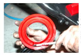
Index the upper part of the spring first and then swing the lower arm up to the spring. Rotate the spring cushion until the cushion will index with the spring. Use a floor jack under the lower control arm to help hold the arm close to the spring. The floor jack should be positioned towards the ball joint side, not directly under the spring pocket.
