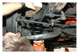
6.Raise the upper arm and spindle assembly up and slide a 2x4 up between the frame and upper arm. This will hold the assembly out of the way so you can work on the lower.
