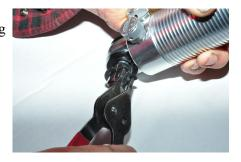
13. Remove the bar by tapping it out of the bushing with a dead blow hammer. If you have a small press you can use that.
