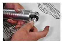
15. The steel sleeve will push into the bushing fairly easy. Push the sleeve in till it bottoms out with the bushing.
