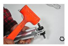
14. Next install the steel sleeve in the bushing, place grease inside the bushing and around the pin. We recommend synthetic grease like NEO Z-12, however any water resistant synthetic grease will work.
