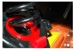
Slowly raise the floor jack and slip the spring into the spring cushion. Sometimes you may need a pry bar to help guide the spring into the cushion.
