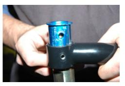
9. After both bushings are pressed in, install the inner white plastic sleeves. Lubricate the inside of the sleeve where the shaft will ride and the inside of the blue housing. We recommend water repellant synthetic grease. Boat hub grease can be used also. You may have to slightly tap the insert into the bushings.
