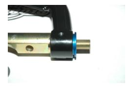
4. When both bushings are press out 1/8 of an inch, slide the shaft to one side, place one of the shims provided in your kit between the white plastic inner thrust washer and the shaft. You will only install the shims on one side.
