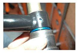
3. Place the control arm with the housing in the press so you can press against the shaft and push the blue bushing out.
