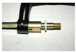
8. Press the blue bushing into the housing.
