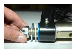
11. Re-install the upper control arm and align.
