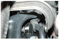
Note: When you reinstall the stud in the frame with the new upper arm. Make sure the stud is in the upper arm shaft, use a drift punch and drive the stud back into the frame.
