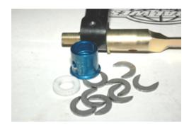
6. Slide the shaft out of the control arm and flip the shaft so the words engraved on the shaft saying (offset) are towards the engine. Note: The words should not be upside down looking at the top of the arm. You are now ready to reinstall the bushings.
