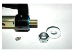
2. Locate a tube or housing of some kind that fits around the blue bushings in the arm.
