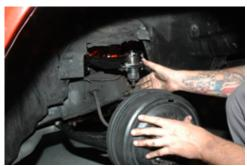
After completing the upper arm installation an alignment will be required. The following specifications will only work with Global West control arms. They will not work with stock control arms.
