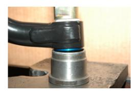
You will only be able to press about 1/8 inch before the shaft will bottom out on the arm. Press both bushings out of the arm 1/8 of an inch.
