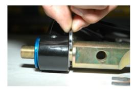
5. Place the arm back into the press and press the bushing with the steel shim out another 1/8 of an inch. Remove the arm from the press and slide the shaft up so you can install another shim against the previous. You will continue this process until all 8 shims are used. The bushing will then come out.
