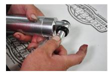
16. The steel sleeve will push into the bushing fairly easy. Push the sleeve in till it bottoms out with the bushing.
