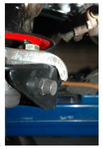
Slowly raise the floor jack and slip the spring into the spring cushion. Sometimes you may need a pry bar to help guide the spring into the cushion.
