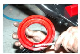
will index with the spring. Use a floor jack under the lower control arm to help hold the arm close to the spring. The floor jack should be positioned towards the ball joint side, not directly under the spring pocket.
