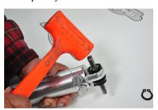
16.Next install the steel sleeve in the bushing, place grease inside the bushing and around the pin. We recommend synthetic grease like NEO Z-12, however any water resistant synthetic grease will work.
