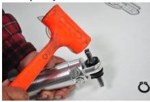
16. Next install the steel sleeve in the bushing, place grease inside the bushing and around the pin. We recommend synthetic grease like NEO Z-12, however any water resistant synthetic grease will work.
