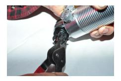
15. Remove the bar by tapping it out of the bushing with a dead blow hammer. If you have a small press you can use that.
