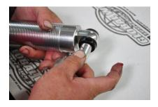
17. The steel sleeve will push into the bushing fairly easy. Push the sleeve in till it bottoms out with the bushing.
