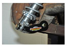
Adjusting the ride height is done by rotating the adjusting nut just below the spring. A spanner wrench included in your kit. The adjusting nut below the coil spring seat is a jam nut. The ride height is adjusted by turning the spring seat, Up raises the car and down lowers the car. Adjusting the ride height is best done by raining the car by the
