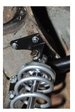
9. Install a ½ x 20 x 3 ½ bolt with a 12mm flat washer through the lower shock mount. The adjusting knobs need to be on the positioned towards the inside of the car.
