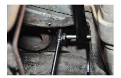
5. The cross member is now lined up against the frame, use a drill with a 3/8 drill bit and drill the frame for mounting the cross member. After the first hole install a 3/8 bolt and nut and just snug.
