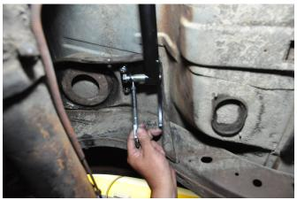
Note: The shock mounts should be loose so they can shift when lining up the bolts for the cross member.
