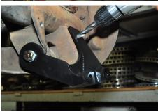
E. Install another  $\frac{1}{2}$  x 20 x 1  $\frac{1}{4}$  bolt with a 12mm flat washer on each side and torque to 70 foot pounds. The final should look like this.
