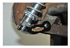
Adjusting the ride height is done by rotating the adjusting nut just below the spring. A spanner wrench included in your kit. The adjusting nut below the coil spring seat is a jam nut. The ride height is adjusted by turning the spring seat, Up raises the car and
