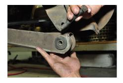
7. Install one of the new lower shock mounts using a new  $\frac{1}{2}$  x 20 x 4 inch bolt and one 12mm flat washer. Slide the bolt through the new lower shock bracket and differential. Install a 12mm washer and a  $\frac{1}{2}$  x 20 lock nut on the other side.
