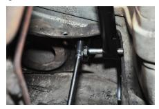
5. The cross member is now lined up against the frame, use a drill with a 3/8 drill bit and drill the frame for mounting the cross member. After the first hole install a 3/8 bolt and nut and just snug.
