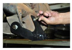
8. Install the shocks starting with the upper mount. Use a  $\frac{1}{2}$  inch x 20 x 3  $\frac{1}{2}$  inch long bolt with a 12mm flat washer and
