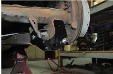
D. Use a drill with a  $\frac{1}{2}$  inch drill bit and drill a new hole through the differential lower arm mount.
