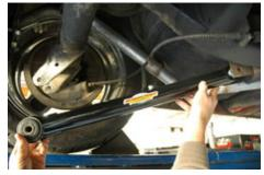
9. On a Moser rear end you will have to remove part of the panhard rod bracket that is welded to the axle tube. The photo shows what is required. The welded bracket is in the way of the coilover shock mounting support clamp. A couple of inches are generally required. It could vary!
