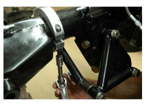
18. Next tighten down the clamps and tighten down the ½ inch bolt holding the short tube.
