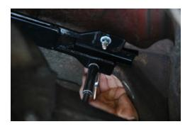
20. Once the cross member is bolted in, use a ½ inch drill motor with a ½ inch drill and drill an additional bolt hole through the frame. One on each side of the cross member.
