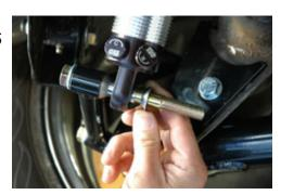
23. Tighten down the  $\frac{1}{2}$  inch bolt holding the shock to 70 foot pounds.
