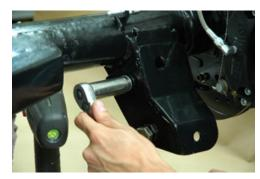
Now install the tubular support bracket. Use a  $\frac{1}{2}$  x 20 x 2  $\frac{1}{2}$  bolt with flat washer and slide it through the mount. Use a thick wall  $\frac{1}{2}$  inch flat washer with a lock nut and slightly run the nut down a few threads just to hold the bracket in place.
