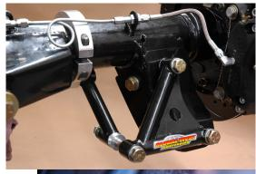
19. Now install the upper cross brace to the frame. The shocks should already be removed. The brace will fit along the top. Install new hardware supplied in your kit. The brace will tuck up into the channel of the frame between the shock mounts.
