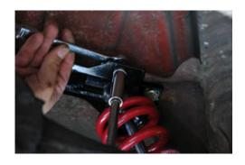
22. Installing the lower portion of the shock. Locate a 5 inch long ½ inch bolt and slide it through the tubular lower mount. Install one of the tapered shock mount spacers first on the bolt. The taper goes towards the shock. Slide the shock onto the bolt and then another tapered spacer. (See photo).
