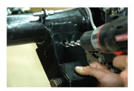
13. Using a ½ inch drill and ½ inch drill bit, drill the side mounting bolt hole. Make sure the bracket is tight up against the rear end mount. You may want to clamp it.
