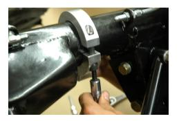
16. Get the one of the short straight tubes and a 2 x ½ x 20 bolt with lock washer and flat washer, and slide bolt through the aluminum clamp. See photo – next thread the bolt into the short straight tube (one end is threaded). Do not tighten down yet, just run the bolt down till you have some resistance on the tube. The tube will need to pivot slightly for alignment.
