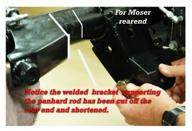
10. Locate in your kit one of the 5/8 bolts with a flat machined into it. Slide a flat washer on it and install the bolt through the correct (right or left) shock mounting bracket supplied in your kit. See photo --
