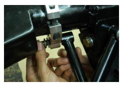
17. Next use one of the 5 ½ inch long ½ inch bolts and slide it through the triangle bun. You can use the base of the coilover shock to space the bracket. In the photo we used a spacer. Line the other side of the straight tube up with the bolt. You will have to move the clamps to position the straight tube so the bolt slides through. Temporary tighten down the bolt.
