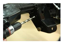
Use one of the  $\frac{1}{2}$  inch bolts, one flat washer and one  $\frac{1}{2}$  x 20 loc nut, Tighten down the bracket 70 foot pounds
