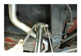
rear end side. New hardware is supplied. The front of the arm has a special bearing in it that allows for pivot. Install the front of the arm on the frame first. It has a spacer on each side of the bearing. They are already installed in the arm. Make sure the spacers don't fall out during installation; you will need them for proper spacing in the frame bracket. Tighten to 120 foot pounds.
