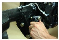
14. Next slide the bottom of the tubular bracket over to the index hole in the new bracket. You may or may not need spacers. If so they are supplied in your kit. You want the bracket to be flat. Using a ½ inch x 20 bolt and flat washer, slide the bolt through and using a ½ x 20 lock nut tighten down the assembly to 70 foot pounds. You can now tighten the upper bolt as well to 70 foot pounds.
