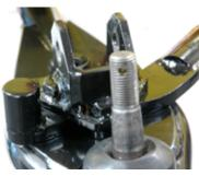
The bolts are 9/16 and  $\frac{1}{2}$ . Install a  $\frac{1}{2}$  inch flat washer and lock nut on the  $\frac{1}{2}$  inch bolts. Install one 9/16washer on each 9/16 bolt and use the 9/16 lock nuts supplied in the kit. Torque all 3 nuts to 70 foot pounds.
