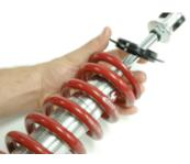
F. The upper shock spring cap slides over the shaft as
