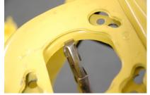
7. If you have ordered a Negative Roll System you will have an upper control arm template for drilling different locating holes. Note: If you did not order a negative roll system no template will be provided however you will have to drill the upper mounting holes out to 9/16 diameter. The original holes are ½ inch diameter. Slide a couple of ½ inch bolts through the template and inner shock tower. Position the new holes so they are below the original, center punch the holes.
