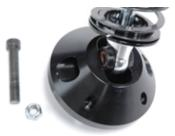
H. Adjust the collar at the bottom of the shock, up until it touches the upper cone for installation. We suggest adjusting the collar up to about 3  $\frac{1}{4}$  inches from the top of the
