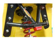
before a measurement can be taken. Adjusting the ride height requires raising the front end off the ground. A spanner wrench (provided in your kit) is used to rotate the adjusting collar. Screwing the collar up on the shock raises the car, down lowers the car. When installed most of the time the collar will be close to the top of the threads on the shock.
