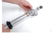
First slide one thin washer over then the bearing and then the last thin washer. Do not lubricate the bearing. The lube will collect dirt over time and stop the bearing from rotating.
