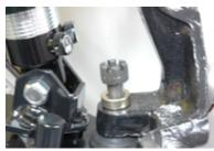
Tighten down the spindles to 80 foot pounds on the lower and 70 foot pounds on the
