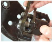
The bolts are 9/16 and ½. Install a ½ inch flat washer and stovelock nut on the ½ inch bolt. Install one 9/16 washer on each 9/16 bolt and use the 9/16-stovelock nuts supplied in the kit. Torque all 3 nuts to 70 foot pounds.
