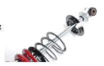
G. Remove the ½ inch bolt from the top shock mount. Install the shock in the mount and slide the ½ inch bolt back through and tighten. 50 foot pounds.
