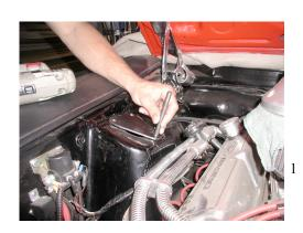
Take the template and align the holes so they locate in the narrow slot where the carriage bolts index. Center punch the inside hole first. Do not center punch all the holes at this time
