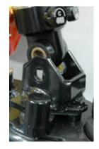
Install as shown and also install the upper ball joint through the spindle.
