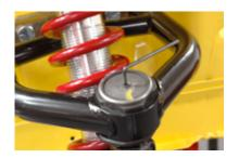
18. Hook up your steering and the sway bar. Many times it's easier to put the sway bar end links on after the cars ride height is set and on the ground.
