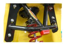
17. After the ball joints are tightened down lubricate the upper ball joint. After you lubricate the ball joint you need to remove the grease fitting and install a plug. This is so the bump stop hits the top of the ball joint flat.
