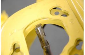
8. If you have ordered a negative roll system you will have an upper control arm template for drilling different locating holes. Note: If you did not order a negative roll system no template will be provided but you will have to drill the upper mounting holes out to 9/16 diameter. The original holes are ½ inch diameter. Slide a couple of ½ inch bolts through the template and inner shock tower. Position the new holes so they are below
