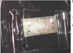
The picture below shows the template in position and center punching the lower holes.
