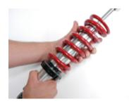
D. On top of the spring you will install a small stepped ring. The ring will index inside the spring.
