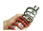
F. The upper shock spring cap slides over the shaft as shown to the right.
