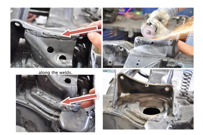
Step 4: Measure 3/8" from the engine side of the upper control arm frame bracket. Using a pneumatic cut off wheel or 4" grinder cut along the top of the upper arm bracket.
