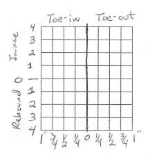
Note: Jounce is when the tire goes up into the fender. Rebound is when the tire drops out of the fender.
