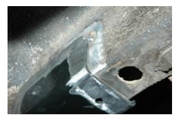
6. After the tacking process is complete, weld the subframes to the rails.
