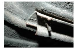
3. Once you finished notching the floor support, the subframe will go up tight against the floor rails. Push the subframe forward on the car so it butts up against the forward floor rail. Mark the floor rails around the subframe so the area can be prepped before welding. In addition you will need to grind the powder coat off the end of the rear box and front plate on the subframe for proper weld penetration.
