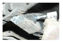
5. After you have prepped the frame and subframe. Hold the subframe up into position and tack the subframe to the frame rails. Make sure the forward portion of the subframe intersects the forward two rails and the subframe. Notice the subframe does not cover up the frame rail holes.
