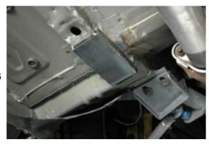
Hold the subframe up and position it so you can mark the areas for buffing off the paint on the floor. Buffing off the paint will insure good welds. You will notice the rear of the subframe will fit matching the slope of the rear bulkhead. Align the plate so the edge of it contacts the main square portion of the rear bulkhead. THE SUBFRAME SHOULD APPEAR TO BE PARALLEL TO THE FACTORY FLOOR RAIL.
