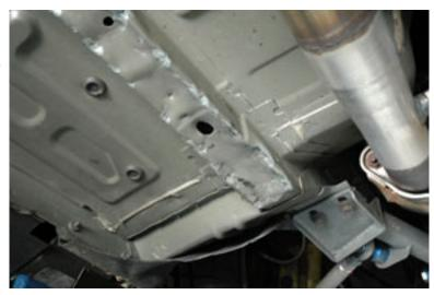
If you run into this (damaged floor) on your car, a 3/16 thick plate must be added to the rail before installing the subframe. This area for the subframe must be flat. Depending on the extent of the damage, the length of the plate will be at least 5 inches long. Make the plate the width of the floor rail. Weld the 3/16 plate over the damged area as shown in the photo.
