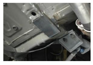
2. Hold the subframe up and position it so you can mark the areas for buffing off the paint on the floor. Buffing off the paint will insure good welds. You will notice the rear of the subframe will fit matching the slope of the rear bulkhead. Align the plate so the edge of it contacts the main square portion of the rear bulkhead. THE SUBFRAME SHOULD APPEAR TO BE PARALLEL TO THE FACTORY FLOOR RAIL.
