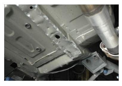
If you run into this (damaged floor) on your car, a 3/16 thick plate must be added to the rail before installing the subframe. This area for the subframe must be flat. Depending on the extent of the damage, the length of the plate will be at least 5 inches long. Make the plate the width of the floor rail. Weld the 3/16 plate over the damged area as shown in the photo.
