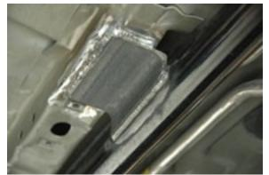
Weld the angle plate to the floor rail and subframe.
