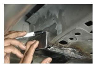
6. After welding the main subframes in place, weld the rear angle plate to the frame. See photo above.
