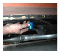
6. The final bushing on the passenger side is the radiator core support. It is one of the 2 –inch diameter male bushings with a 1/2 –inch hole. This bushing installs the opposite as the others. The step part of the bushing goes up through the radiator core mount. Slide the bushing into place and lower the body back down onto the frame.
