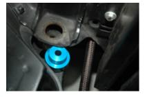
7. Install the female portion of the bushings located at the firewall and radiator core support. The bushing indexes on the step of the installed male bushing and sandwiches the frame. Basically when the assembly is tightened, the bushing halves will lock the frame in position so it cannot slip. The additional spacers in the kit go between the
