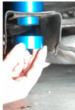
8. Install the female portion of the back bushing located with the subframe kit. Install using a 5/8 x 4-inch long bolt with a 5/8-lock washer and 5/8 flat washer. Do not tighten yet.
