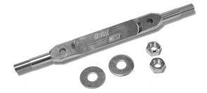
The 709 shaft will fit Global West tubular upper arms CTA-79 series, CTA-42 series and stock control arms using rubber, polyurethane, or Global West Del-a-Lum bushings.
